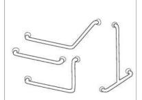
When marking out the grab rails, use centre base holes of flange protector.
